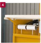
1 Compact your waste and eject the finished bale. 2 Remove and store the bale until collection. 3 The baler has a simple control panel and is equipped with easily understood pictograms. 4 The strap rolls are easy to replace in front of the machine.
